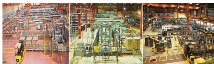
Bottling Line 2: 36000 bottles per hour
